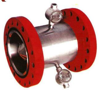
The Custody Transfer series Inline Turbine Flow meters are designed to provide high accuracy liquid flow measurement under the exacting conditions encountered in the Oil Industry. Being capable of achieving ±0.15% linearity or better, over a specified flow range- they are specifically intended for use in fiscal or custody transfer applications. CT flow meters are specially designed to minimize viscosity effect in order to preserve the linearity over a flow range.
